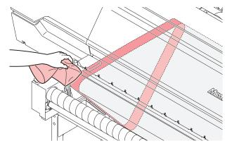
**2** Feed the belt by specifying the count in [Maintenance] > [Belt Maintenance] > [Belt Cleaning].
