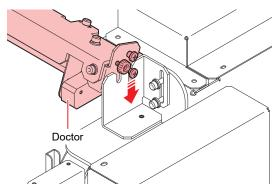
(4) Adjust the doctor adjustment plate height to around the level where the doctor blade touches the feeding belt, then secure it in place.
