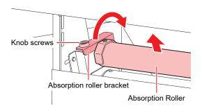
**Q** Remove the absorption roller from the machine.
