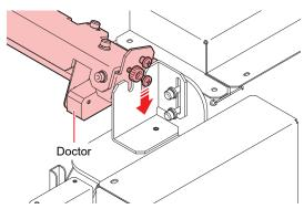
(4) Adjust the doctor adjustment plate height to around the level where the doctor blade touches the feeding belt, then secure it in place.
