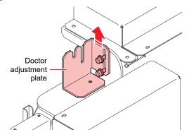
(2) Loosen the doctor guide blocks (at each end) enough to allow the doctor to move up and down under its own weight.
