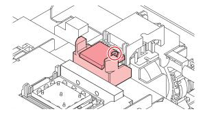
10 Check to confirm that the absorber is not lifting or curved.
